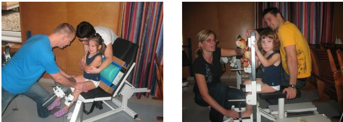
Figure 3: Maximum voluntary torque measurement in knee extension (left) and ankle plantar flexion (right)
